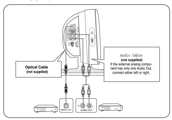
Connect the Digital Input (OPTICAL) to the Digital Output on the external digital component.
